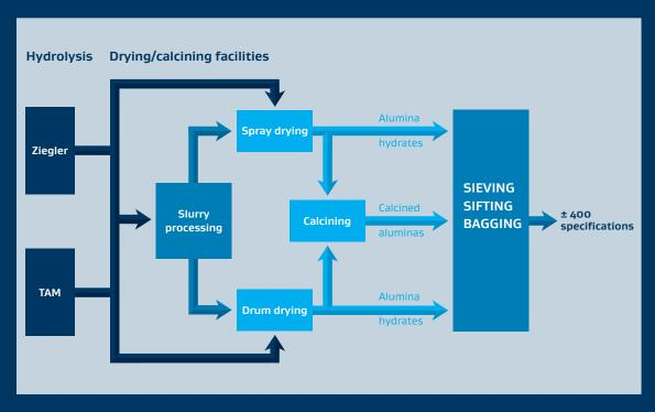
Figure 1: Schematic for the alumina manufacturing process
